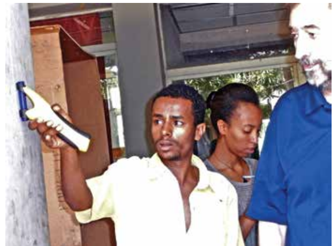
A student uses the Zircon m40 to locate vertical bars in a concrete column
