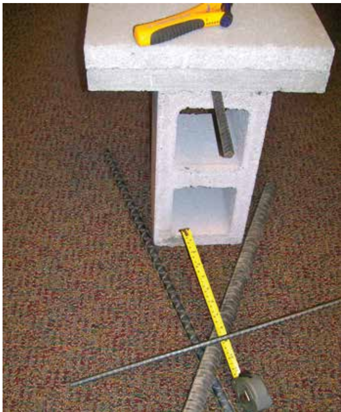
A simple test setup to evaluate the metal locator
