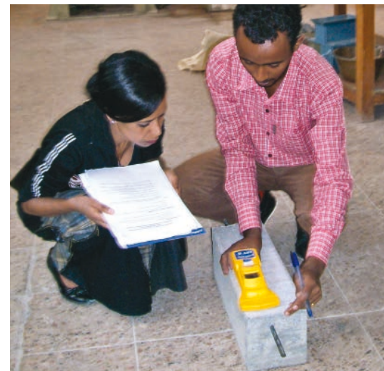
Students test a beam with the MT6 metal locator. The tool is used to locate rebar in concrete.
