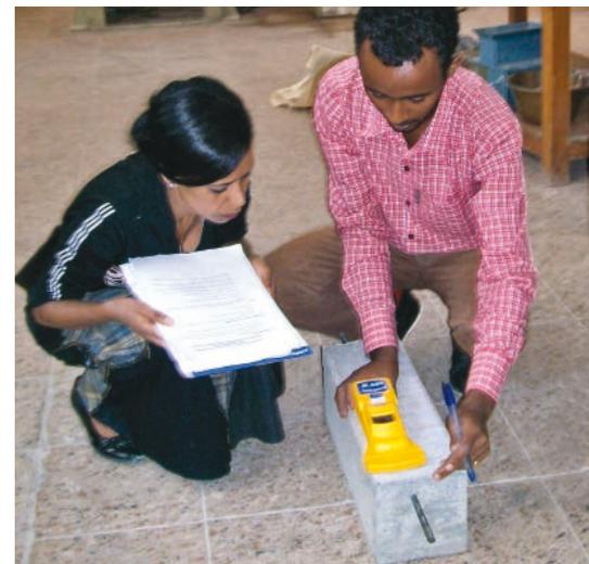
In most cases, the contractor will only occasionally use the metal locator. Unlike forensic engineers that need detailed information about the reinforcement, the contractor usually needs equipment that is easy to use and will answer basic questions, such as was the reinforcement installed or how can I avoid the reinforcement if coring or drilling a hole into the concrete?
